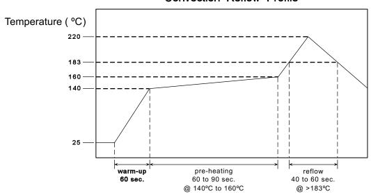
**NOTE:** The CS-300 should not be subjected to a wash process that will immerse it in solvents. NO CLEAN is the recommended procedure. The CS-300 has been designed for pick and place reflow soldering. The suggested reflow profile is shown above. The CS-300 may be reflowed once, and should not be reflowed in the inverted position.
