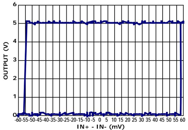
FIGURE 14. HYSTERESIS - 50mV ( $V_+ = 5V$ )
