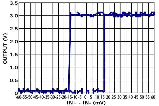
FIGURE 16. HYSTERESIS - 12.5mV ( $V_+ = 3V$ )
