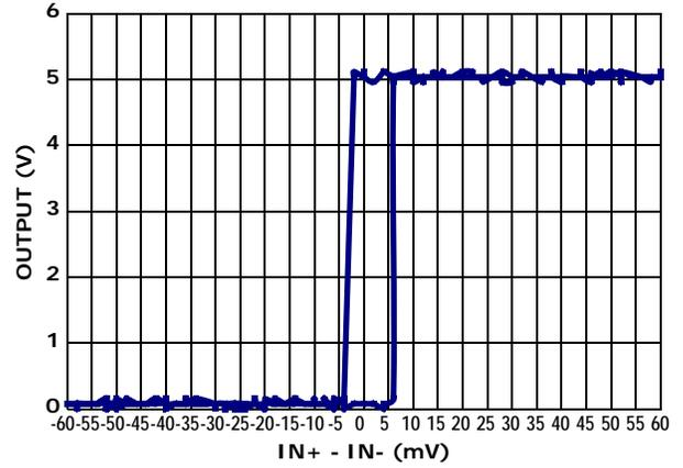
FIGURE 10. HYSTERESIS - 0mV ( $V_+ = 5V$ )
