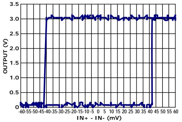
FIGURE 18. HYSTERESIS - 37.5mV ( $V_+ = 3V$ )
