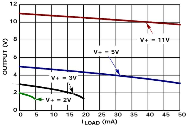
FIGURE 9. COMPARATOR OUTPUT HIGH VOLTAGE vs LOAD
