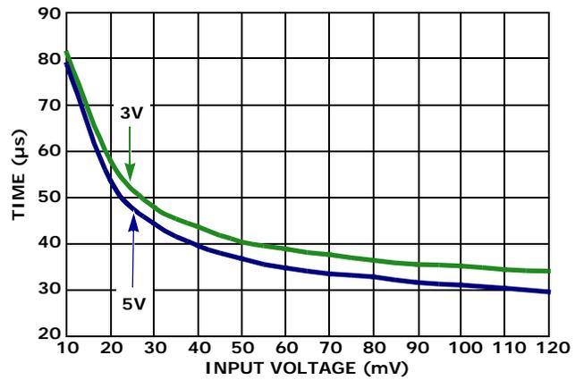
FIGURE 20. OUTPUT RESPONSE TIME vs INPUT OVERDRIVE ( $t_{PHL}$ )
