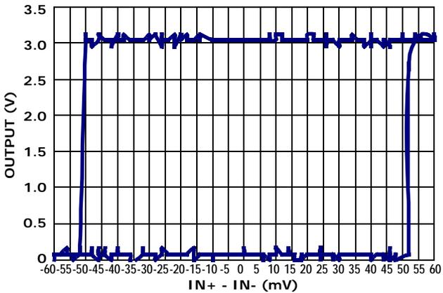
FIGURE 19. HYSTERESIS - 50mV ( $V_+ = 3V$ )
