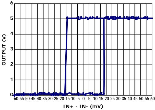
FIGURE 11. HYSTERESIS - 12.5mV ( $V_+ = 5V$ )
