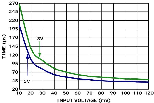
FIGURE 21. OUTPUT RESPONSE TIME vs INPUT OVERDRIVE ( $t_{PLH}$ )
