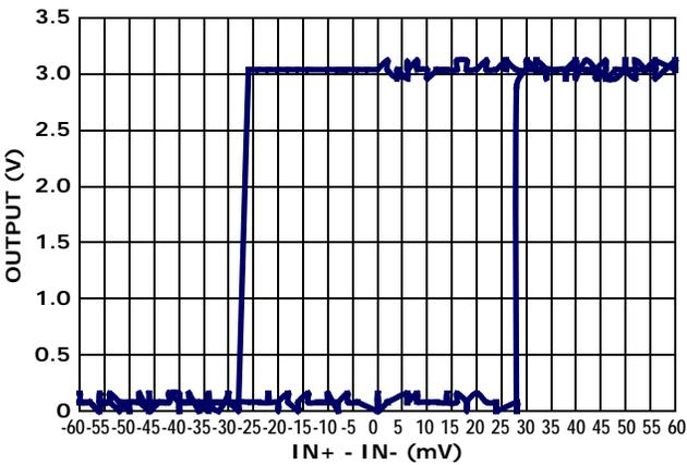
FIGURE 17. HYSTERESIS - 25mV ( $V_+ = 3V$ )
