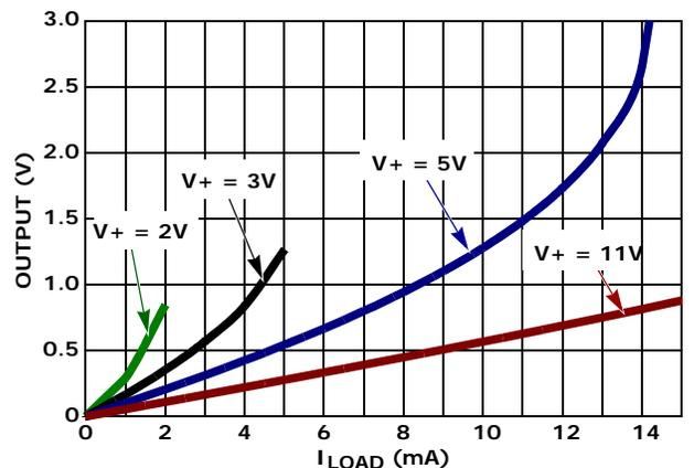
FIGURE 8. COMPARATOR OUTPUT LOW VOLTAGE vs LOAD
