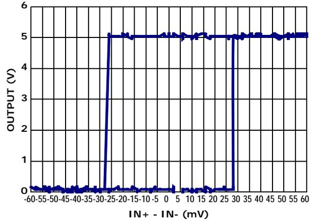
FIGURE 12. HYSTERESIS - 25mV ( $V_+ = 5V$ )
