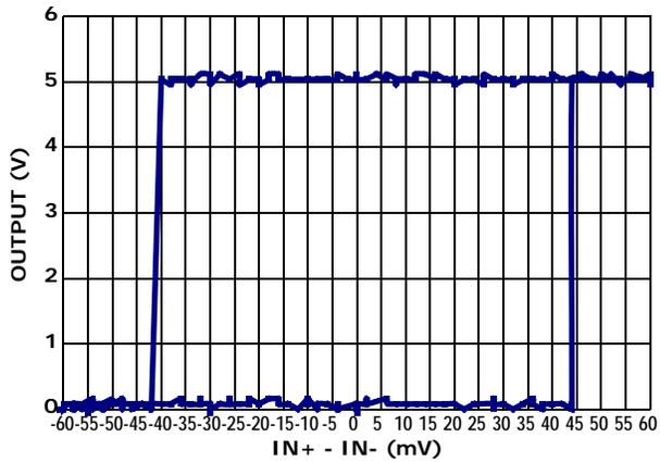
FIGURE 13. HYSTERESIS - 37.5mV ( $V_+ = 5V$ )
