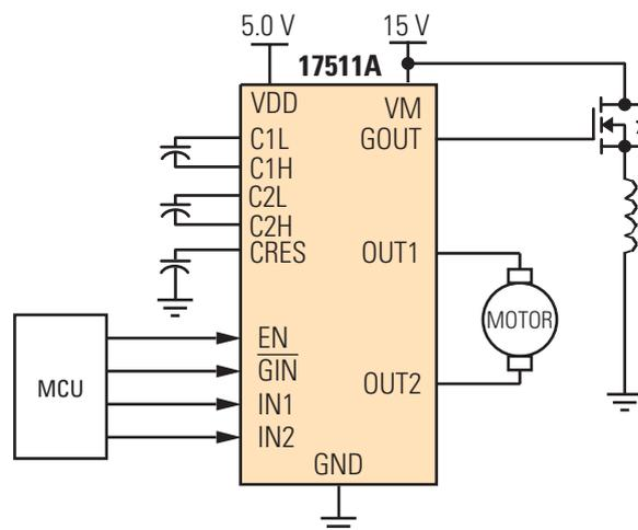
**Figure 1. 17511A Simplified Application Diagram**
