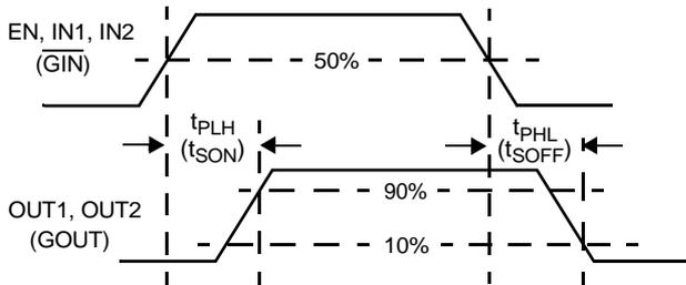
Figure 5.  $t_{PLH}$ ,  $t_{PHL}$ , and  $t_{PZH}$  Timing
