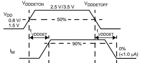
Figure 6. Low-Voltage Detection
