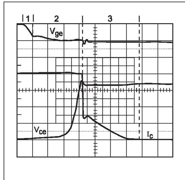
devices, is designed to be relatively high to obtain a lower  $V_{CE(sat)}$ . The lower  $V_{CE(sat)}$  is paid for with a longer current tail, see fig.7, but this price is acceptable because switching losses are negligible because of low switching frequency, compared to the losses during the on phase and during the current regulation. Moreover a very low  $V_{CE(sat)}$  is important to allow the engine to start when the battery voltage is at its lower limit.
