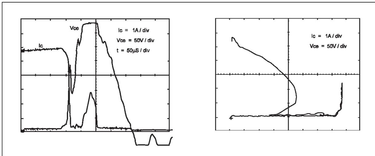
the clamp voltage for the Zener and, if present, the collector-to-emitter capacitance. With a reasonable margin for the current, e.g. 8A, the switch must survive the switch-off without load on the coil secondary side.
