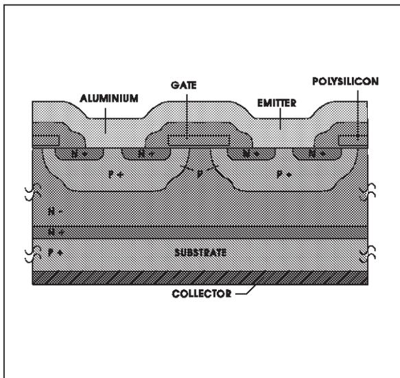
Although their structures are similar, the physical operation of the IGBT is very different from that of the Power MOSFET; the IGBT is a minority carrier device, and its behaviour is closer to that of bipolar transistor. This is due to the p<sup>+</sup> substrate which, during conduction, injects holes in the n<sup>-</sup> region, significantly reducing its resistivity.
