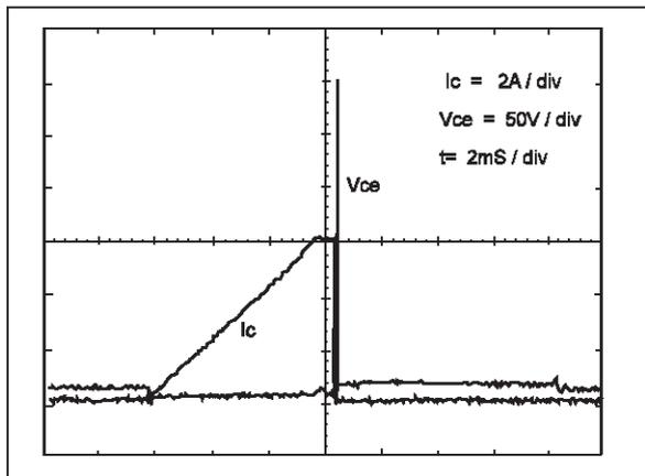
The switch breakdown, which must be never exceeded, must therefore be specified at least 50 V higher than the Zener breakdown to give a reasonable safe margin. Currently IGBTs are available covering a range of  $BV_{CES}$  from 400V to 1500V.
