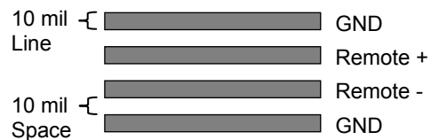
Figure 13 Recommended Remote Diode Circuit Board Interconnect
