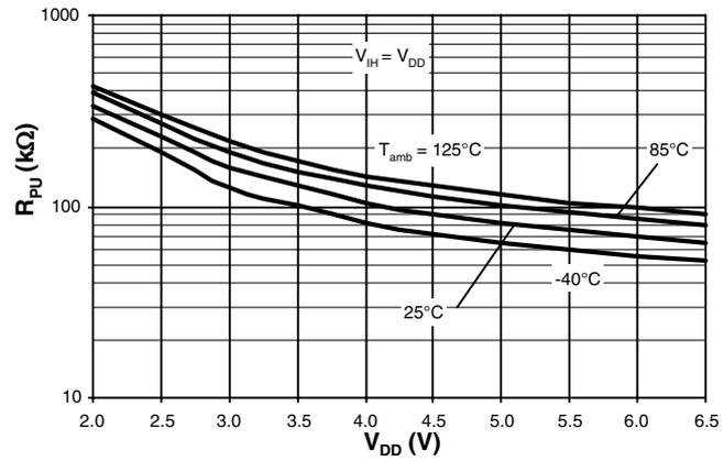
Figure 100. Strong Pull-up Resistor versus  $V_{DD}$
