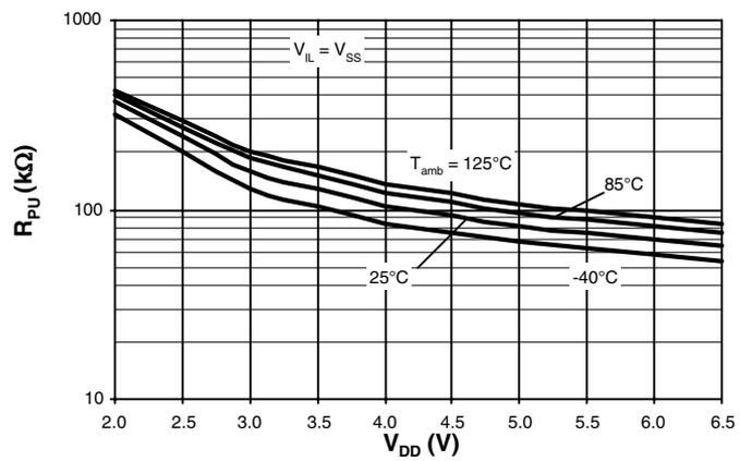
Figure 99. Pull-down Resistor versus  $V_{DD}$
