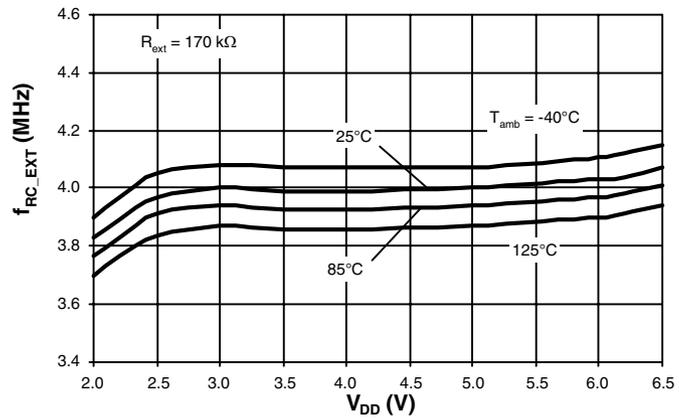
Figure 95. External RC Frequency versus  $T_{amb}$
