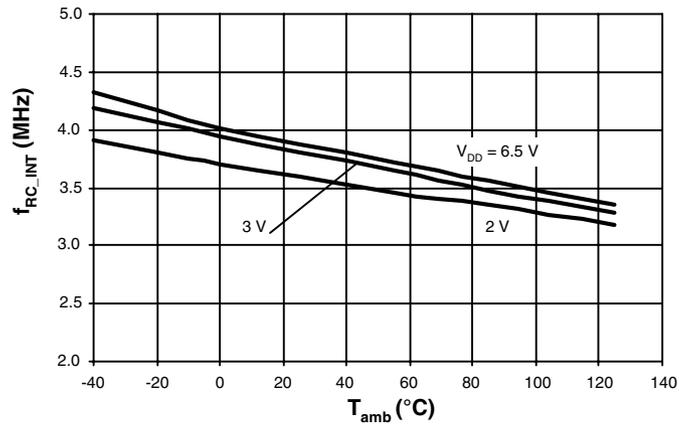
Figure 94. External RC Frequency versus  $V_{DD}$
