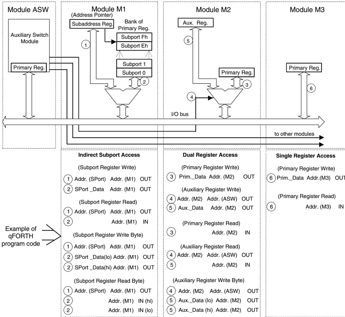
Addr.(ASW) = Auxiliary Switch Module address
