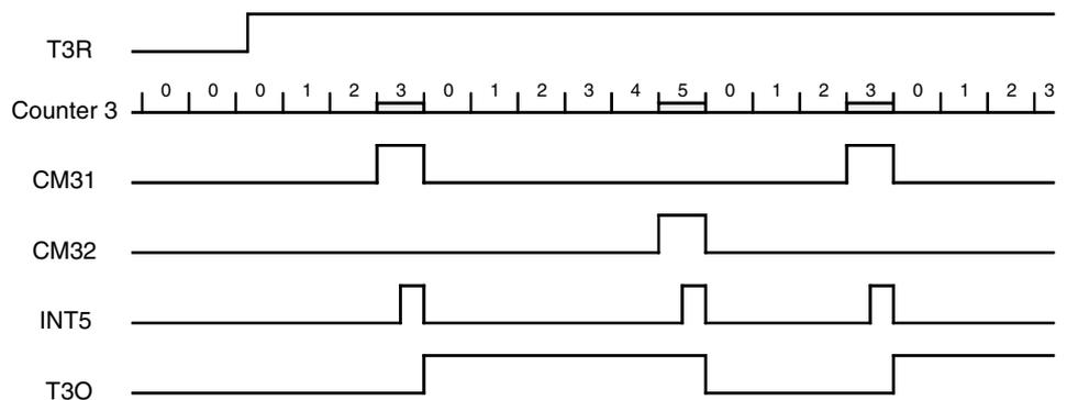
**Figure 46.** Counter Reset with Compare Register 2 and Toggle with Start
