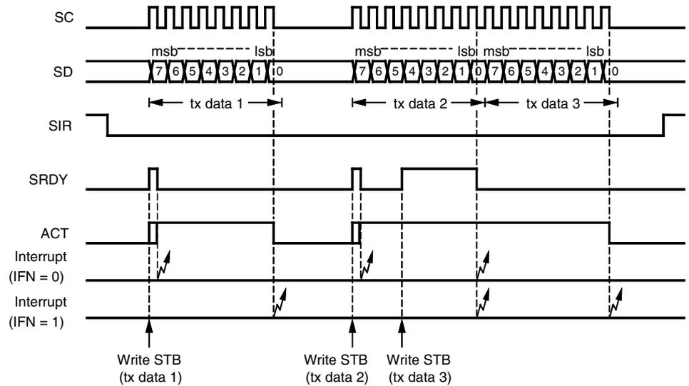
**Figure 60.** Example of an 8-bit Synchronous Receive Operation
