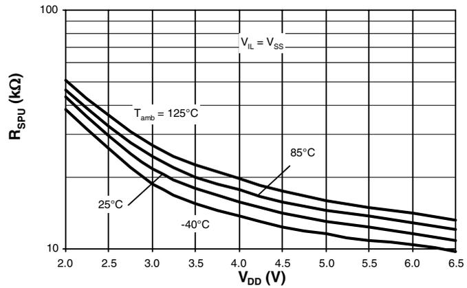
Figure 101. Strong Pull-down Resistor versus  $V_{DD}$
