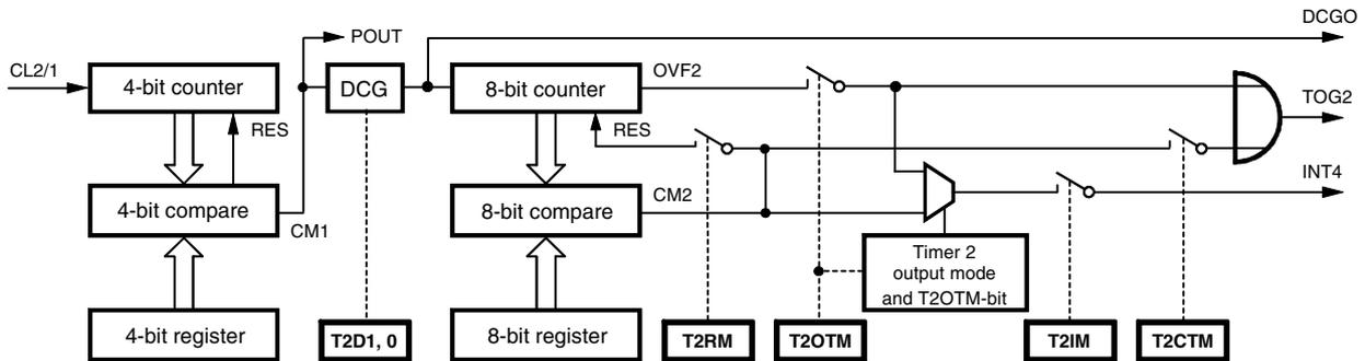
The 4-bit stage is used as programmable prescaler for the 8-bit counter stage. In this mode, a duty cycle stage is also available. This stage can be used as an additional 2-bit prescaler or for generating duty cycles of 25%, 33% and 50%. The 4-bit compare output (CM1) supplies the clock output (POUT) with clocks.
