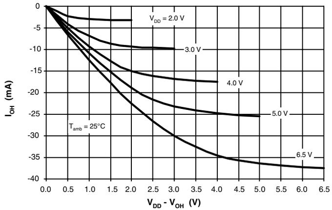
**Figure 103.** Output Low Current versus Output Low Voltage
