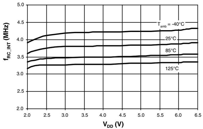
Figure 93. Internal RC Frequency versus  $T_{amb}$
