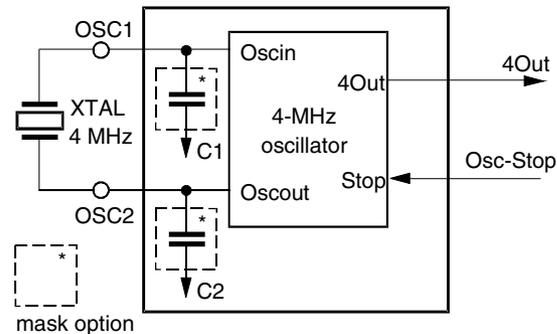
**Figure 18. Ceramic Resonator**
