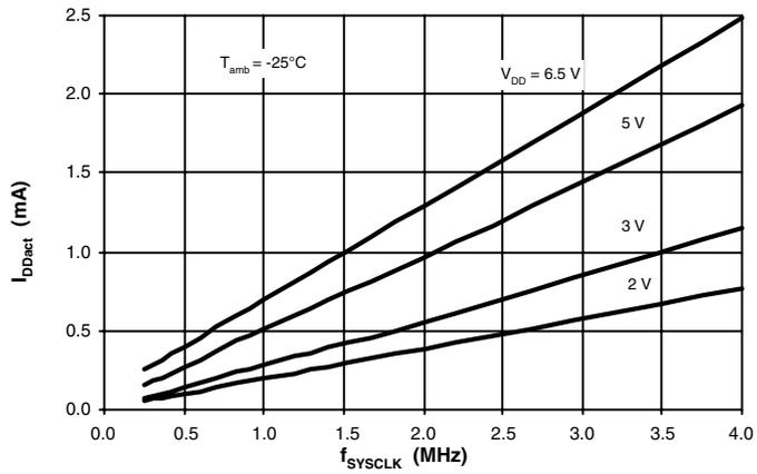
Figure 88. Active Supply Current versus  $V_{DD}$
