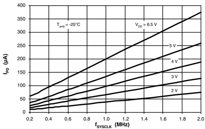
**Figure 90.** Power-down Supply Current versus  $V_{DD}$
