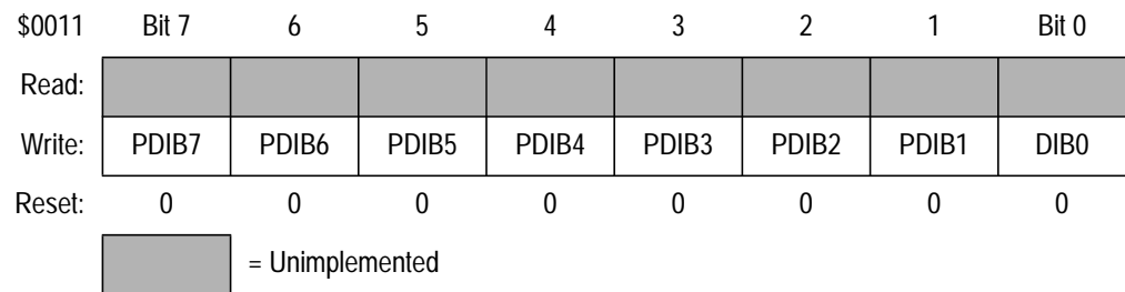
Figure 7-7. Pulldown Register B (PDRB)
