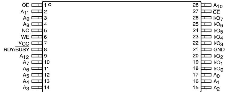
TSOP Package (8mm x 13.4mm) (T13)
