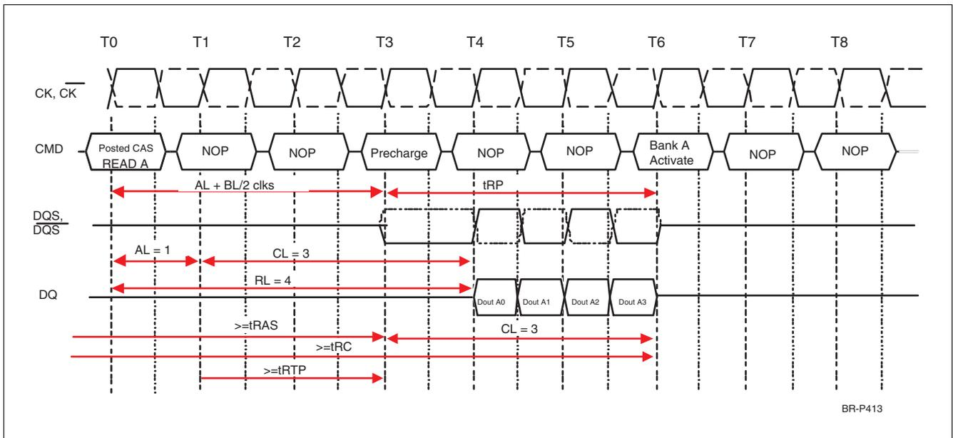
Figure 39 Read Operation Followed by Precharge Example 1:
