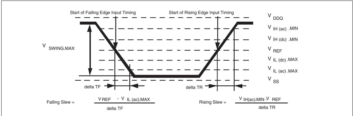
Figure 61 Single-ended AC Input Test Conditions Diagram
