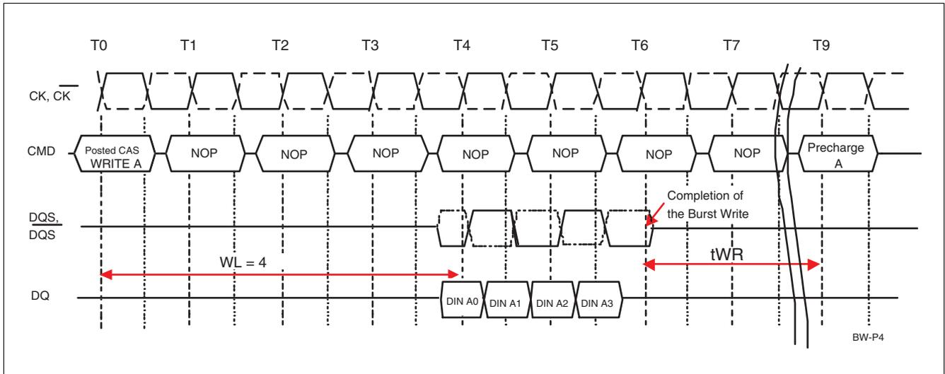
Figure 44 Write followed by Precharge Example 2:  $WL = (RL - 1) = 4$ ,  $BL = 4$ ,  $t_{WR} = 3$
