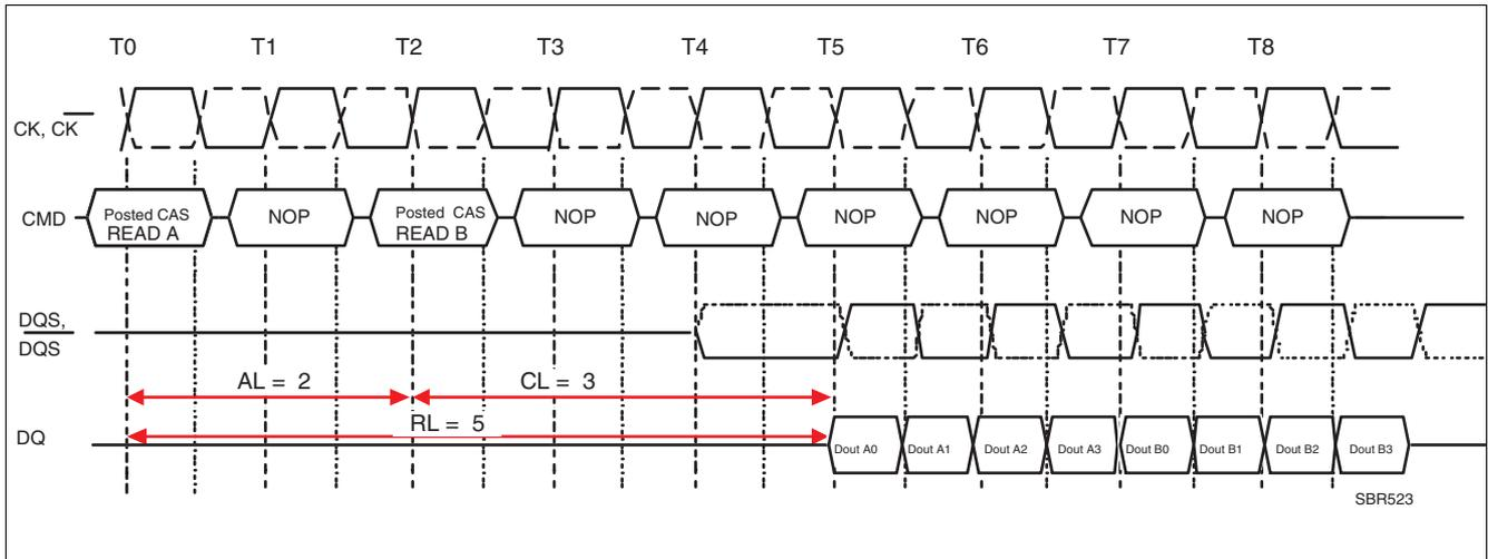
**Figure 27 Seamless Read Operation Example 1: RL = 5, AL = 2, CL = 3, BL = 4**
