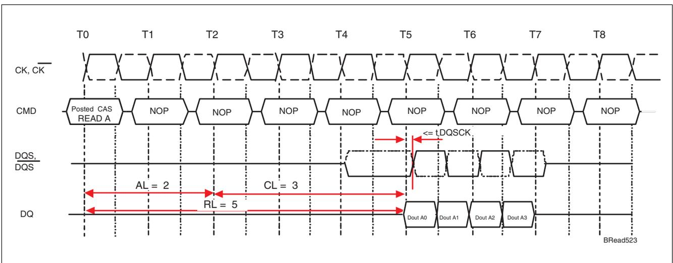
Figure 24 Burst Operation Example 1: RL = 5 (AL = 2, CL = 3, BL = 4)
