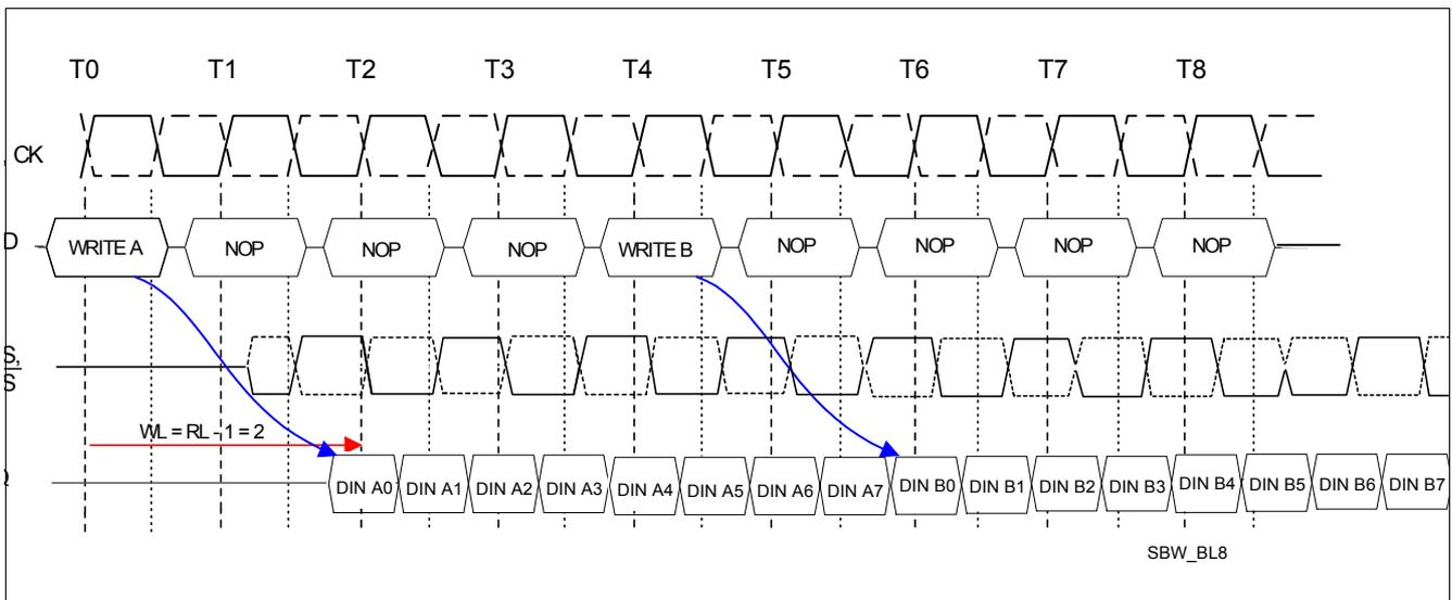
**Figure 34 Seamless Write Operation Example 2:  $RL = 3$ ,  $WL = 2$ ,  $BL = 8$ , non interrupting**
