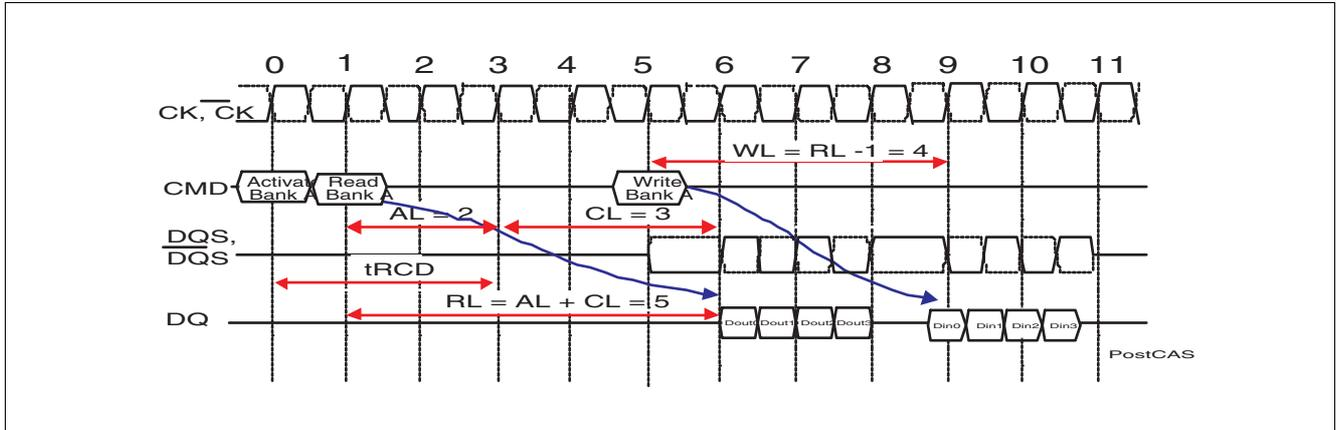
Figure 19 Activate to Read Timing Example: Read followed by a write to the same bank, Activate to Read delay  $< t_{RCD,MIN}$ :  $AL = 2$  and  $CL = 3$ ,  $RL = (AL + CL) = 5$ ,  $WL = (RL - 1) = 4$ ,  $BL = 4$
