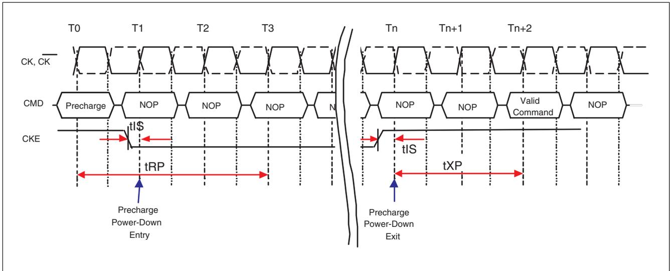
**Figure 56 Precharge Power Down Mode Entry and Exit**
