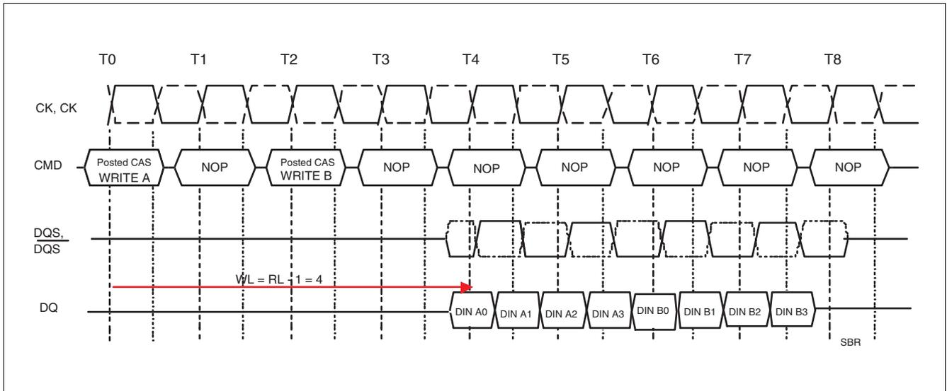
**Figure 33 Seamless Write Operation Example 1:  $RL = 5$ ,  $WL = 4$ ,  $BL = 4$**
