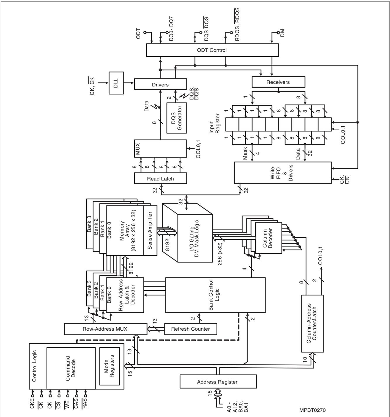
Figure 5 Block Diagram 8 Mbit  $\times$  8 I/O  $\times$  4 Internal Memory Banks
