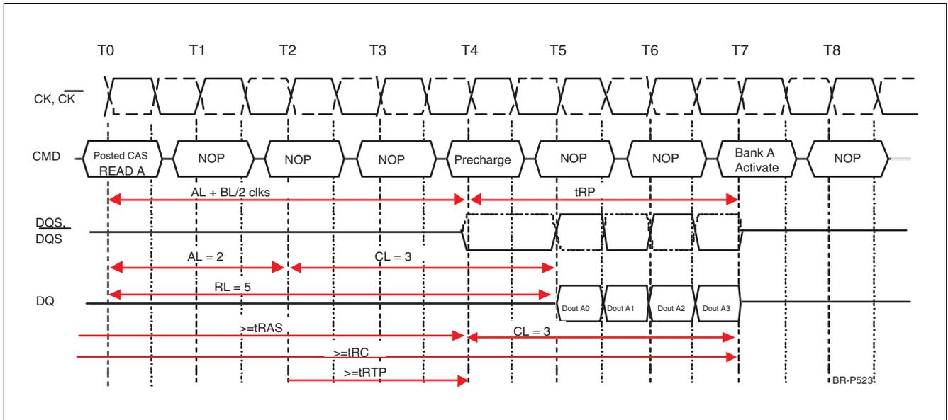
**Figure 41 Read Operation Followed by Precharge Example 3:**
