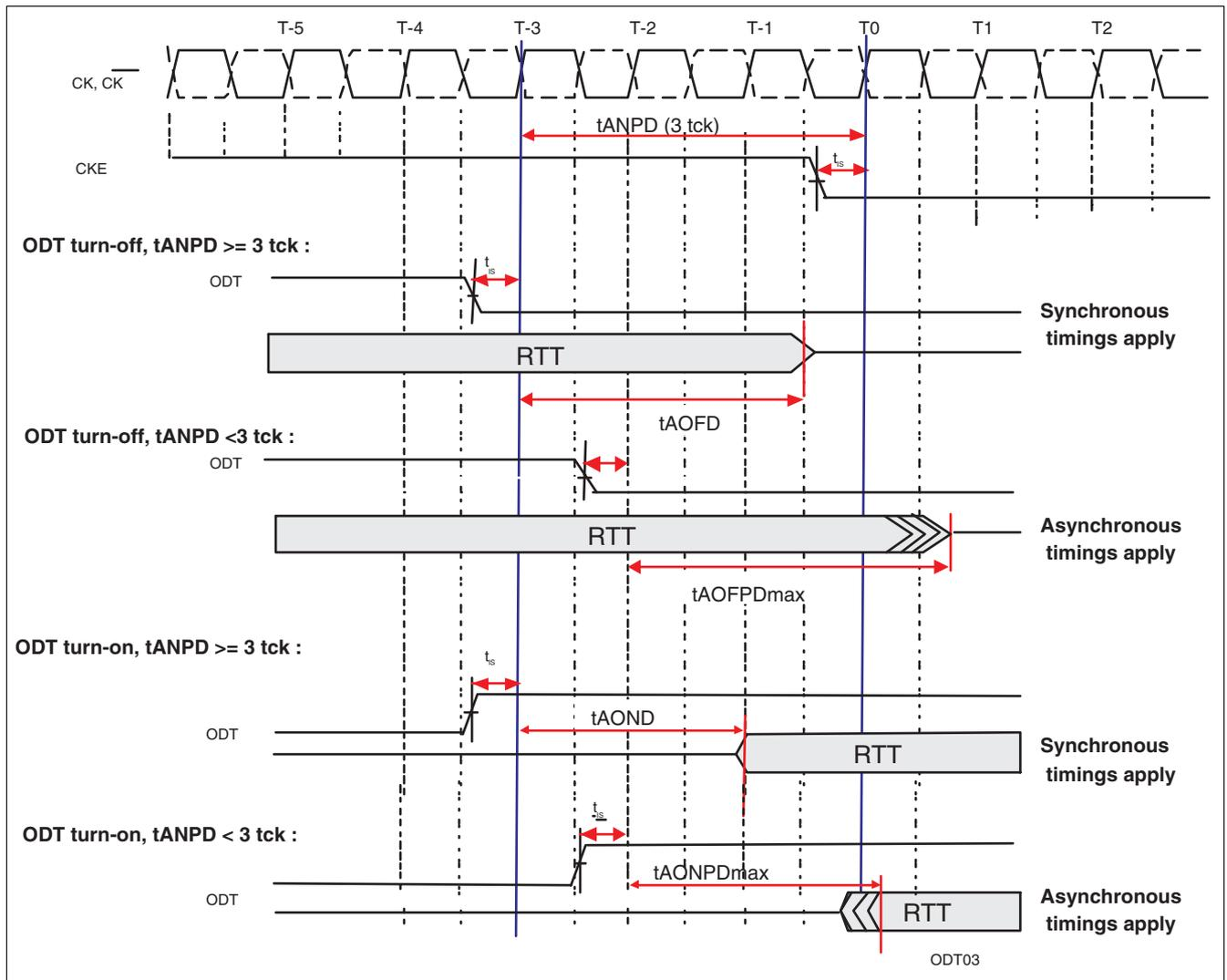
Figure 15 ODT Mode Entry Timing Diagram
