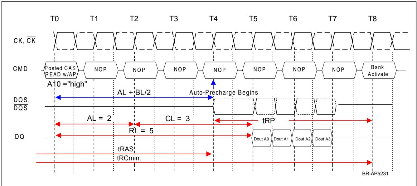
Figure 45 Read with Auto-Precharge Example 1, followed by an Activation to the Same Bank ( $t_{RC}$  Limit):
