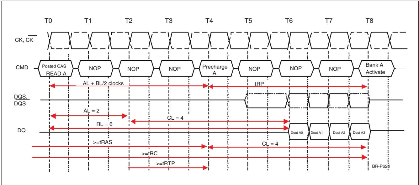
Figure 42 Read Operation Followed by Precharge Example 4:
