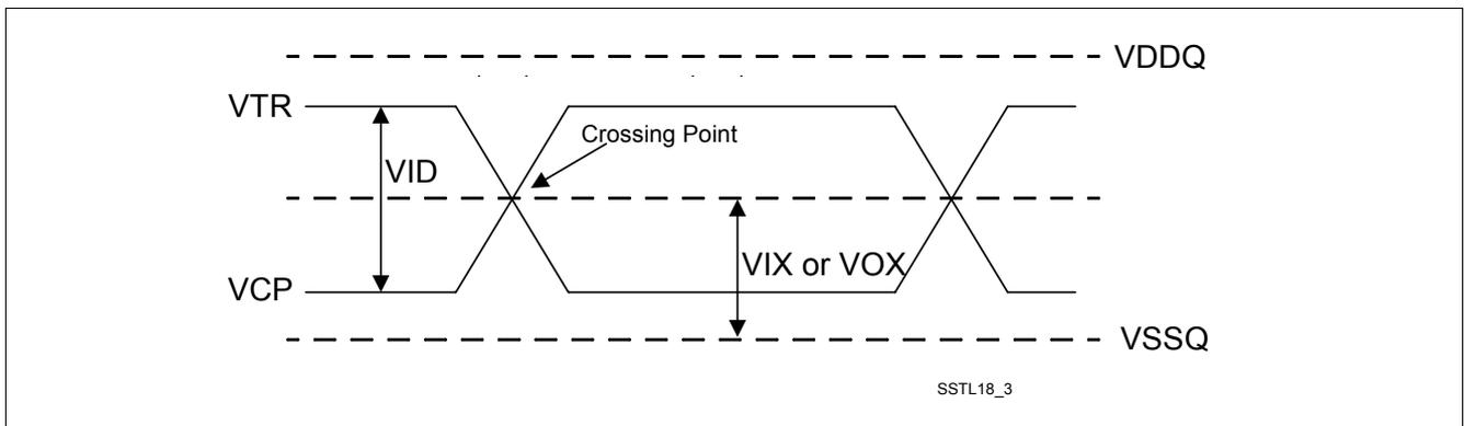
Figure 62 Differential DC and AC Input and Output Logic Levels Diagram
