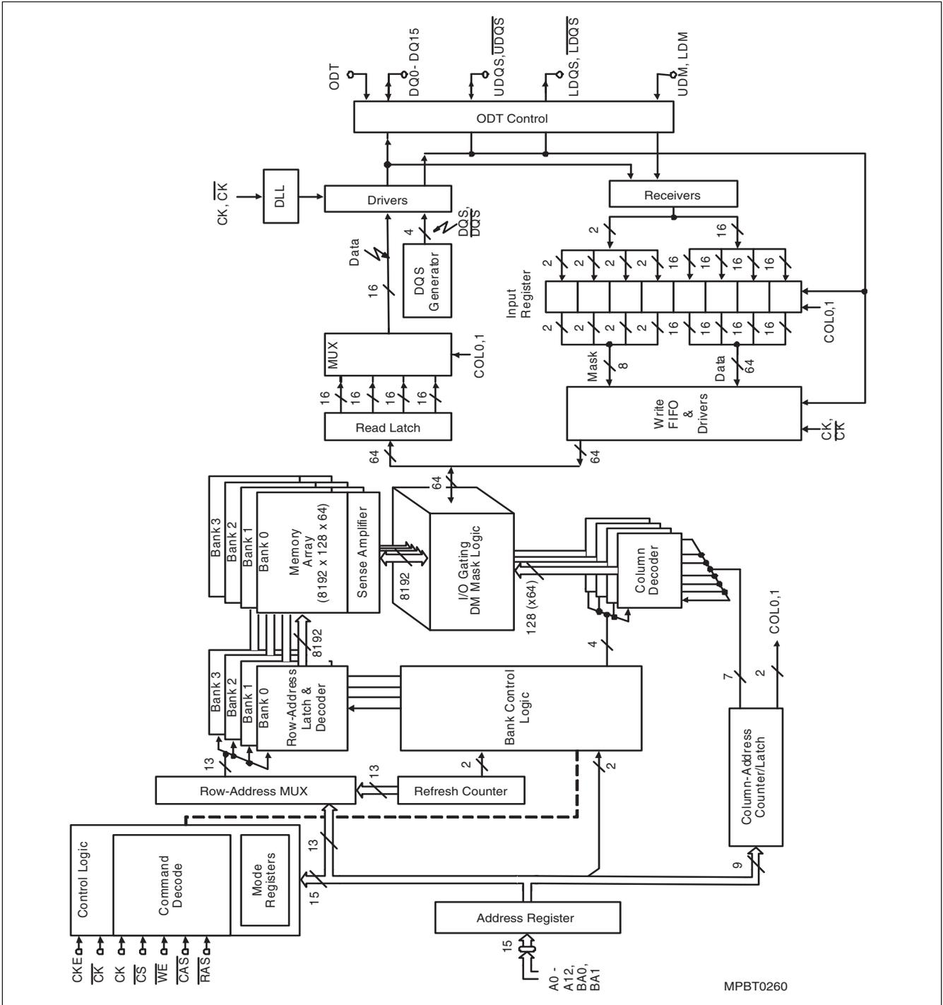
Figure 6 Block Diagram 4 Mbit × 16 I/O × 4 Internal Memory Banks
