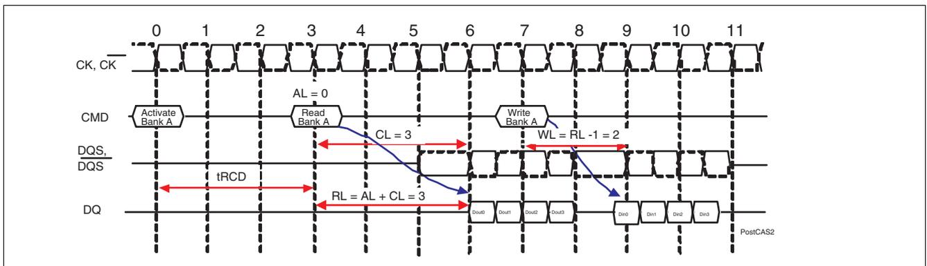
Figure 21 Read to Write Timing Example: Read followed by a write to the same bank, Activate to Read delay  $= t_{RCD,MIN}$ :  $AL = 0$ ,  $CL = 3$ ,  $RL = (AL + CL) = 3$ ,  $WL = (RL - 1) = 2$ ,  $BL = 4$
