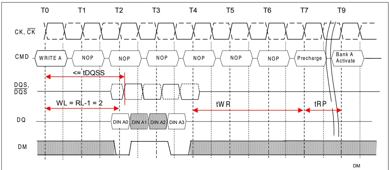
Figure 36 Write Operation with Data Mask Example:  $RL = 3$  ( $AL = 0$ ,  $CL = 3$ ),  $WL = 2$ ,  $t_{WR} = 3$ ,  $BL = 4$
