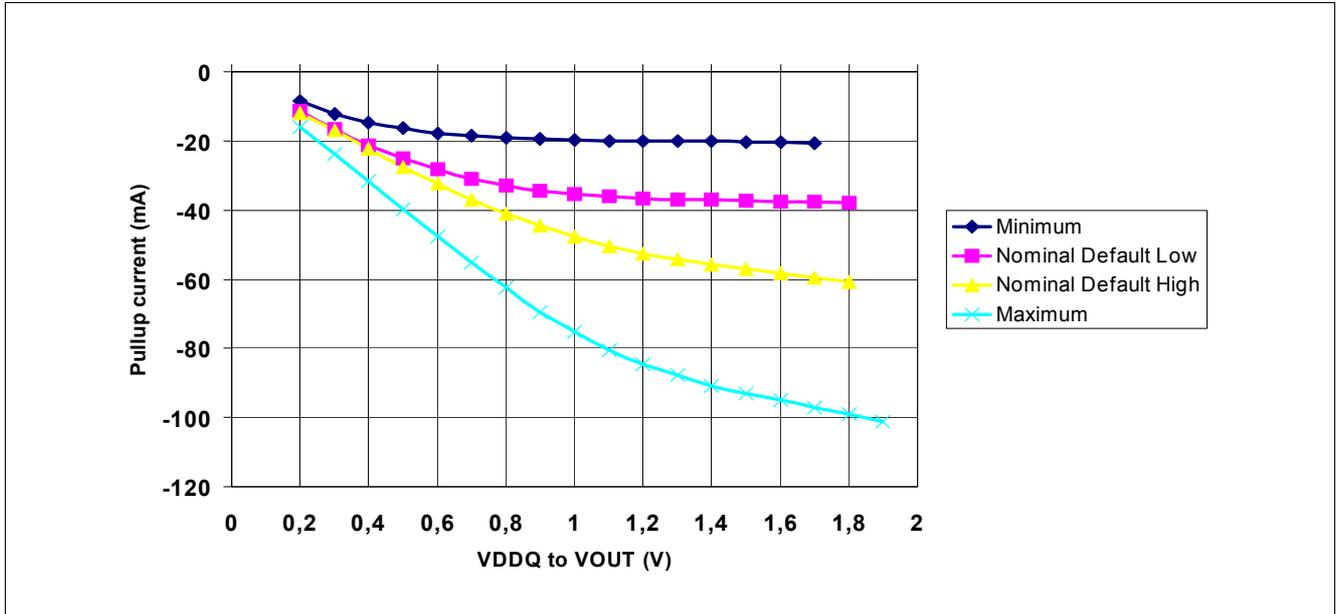
Figure 63 Full Strength Default Pull-up Driver Diagram
