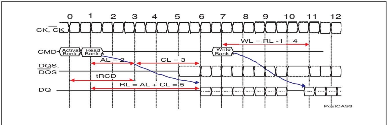
Figure 20 Read to Write Timing Example: Read followed by a write to the same bank, Activate to Read delay  $< t_{RCD,MIN}$ :  $AL = 2$  and  $CL = 3$ ,  $RL = (AL + CL) = 5$ ,  $WL = (RL - 1) = 4$ ,  $BL = 8$
