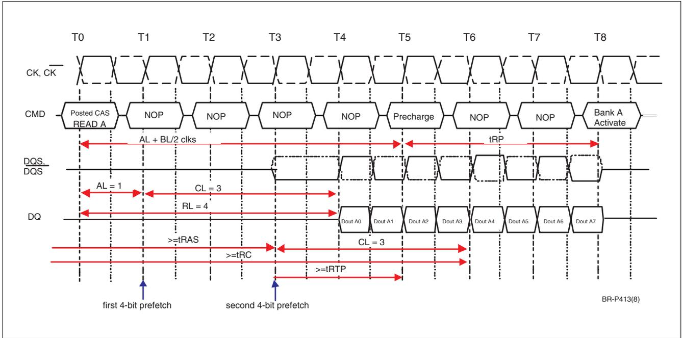
**Figure 40 Read Operation Followed by Precharge Example 2:**
