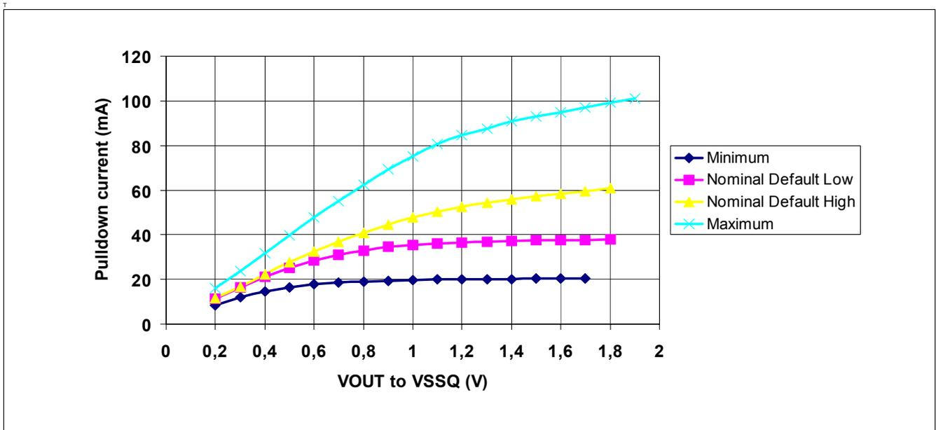
Figure 64 Full Strength Default Pull-down Driver Diagram
