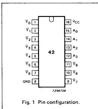
Fig. 1 Pin configuration.
