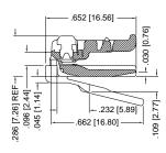
Longer body is ideal for overmolding. Provides more surface area for disconnect/reconnect.
