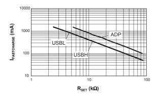
Figure 3: I<sub>FASTCHARGE</sub> vs. R<sub>SET</sub>.
