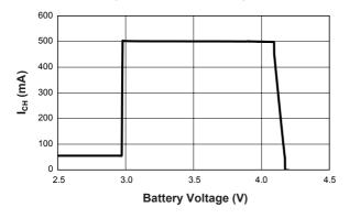
Charging Current vs. Battery Voltage (USBL; USBL = 40.2kΩ)
