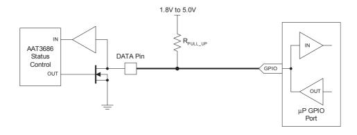
Figure 4: Data Pin Application Circuit.
