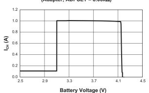
Charging Current vs. Battery Voltage (USBH; USBH = 8.06kΩ)
