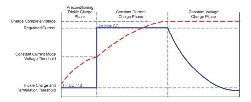
Figure 1: Current vs. Voltage Profile During Charging Phases.
