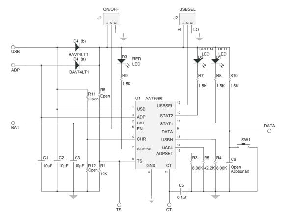
Figure 8: AAT3686 Evaluation Board Schematic Diagram.
