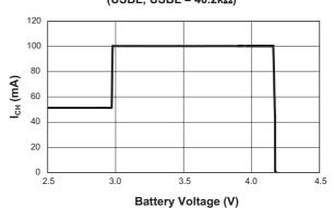
Fast Charge Current vs. Supply Voltage (Adapter; ADPSET = 8.06kΩ)
