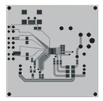
Figure 5: AAT3686 Evaluation Board Component Side Layout.
