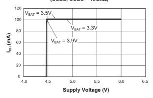
Fast Charge Current vs. Supply Voltage (USBH; USBH = 8.06kΩ)
