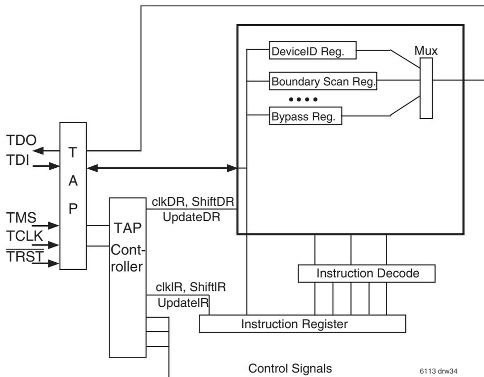
Figure 30. Boundary Scan Architecture
