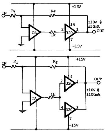
There is a 1k resistor between the output of the operational amplifier and the input of MZ-320. This is optional, but tends to reduce a tendency for oscillation in the op amp output stage. It also provides current limiting at the input under fast slew rate conditions.
