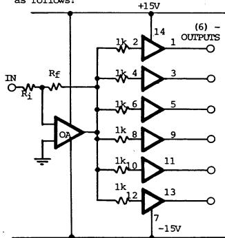
The six seperate outputs have approximately 20dB isolation from a short circuit condition on any one output. Further isolation results if a series resistor at the MZ-320 output(s) is used to source terminate a line.
