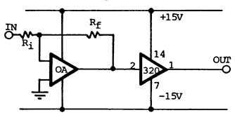
In a data distribution system such as a video distribution amplifier, multiple sections of the MZ-320 can be easily used as follows:
