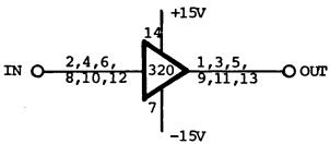
Typical applications are for use as a current booster inside the loop of an operational amplifier. This is shown below, along with the option of paralleling two sections for double the output current. Paralleling more than two sections results in diminishing increase in output current, due to limitations in metalization and internal dissipation.
