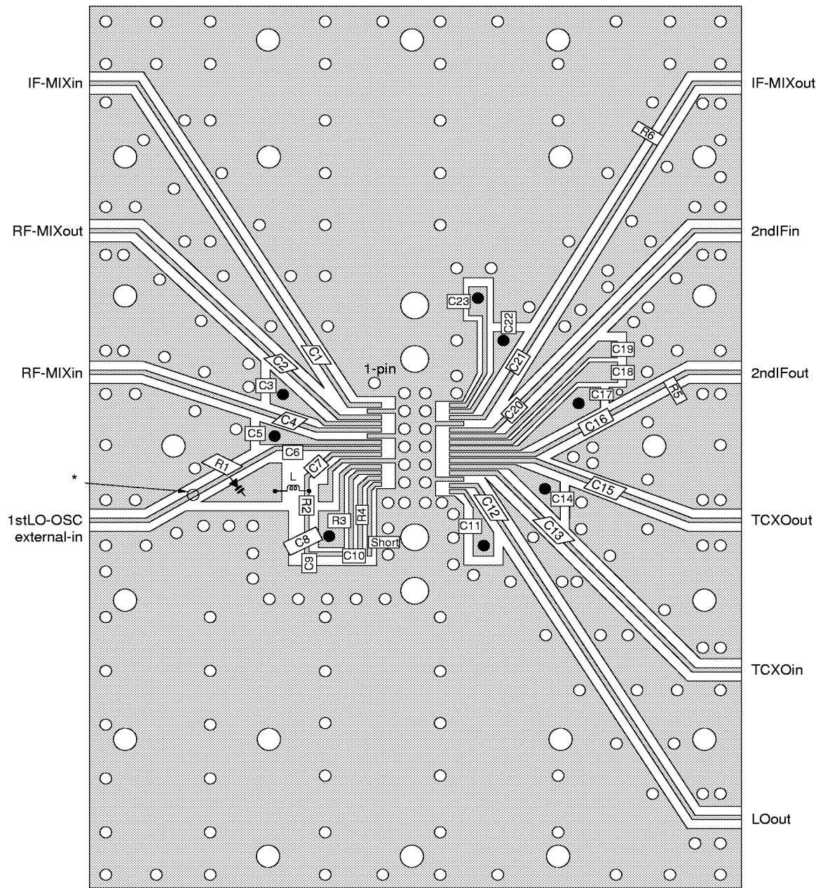
**Notes 1.** 35  $\mu$ m thick double-sided copper clad 63 × 100 × 0.4 mm polyimide board
