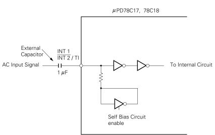
Fig. 2-32 Zero-Cross Detector
