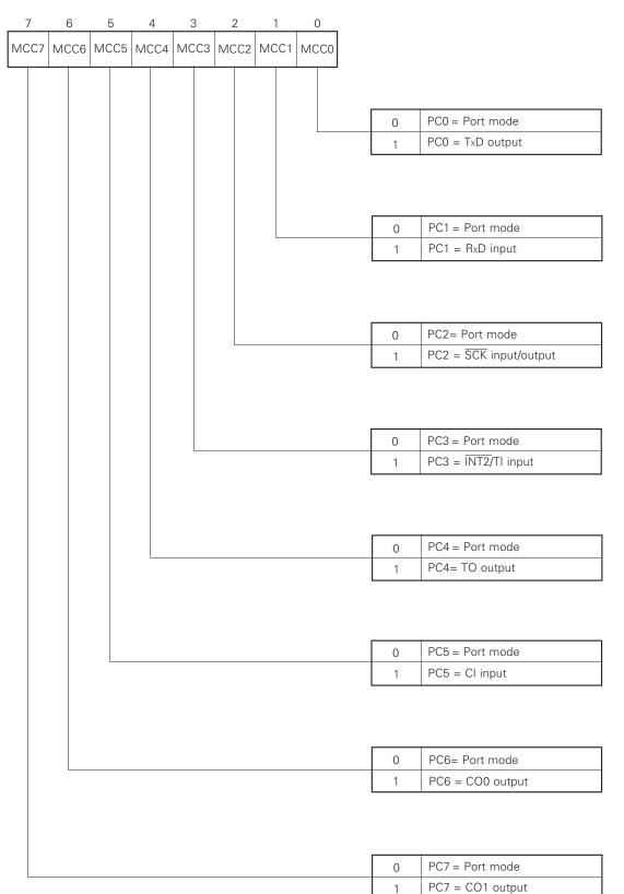
Fig. 2-10 MODE CONTROL C Register Format
