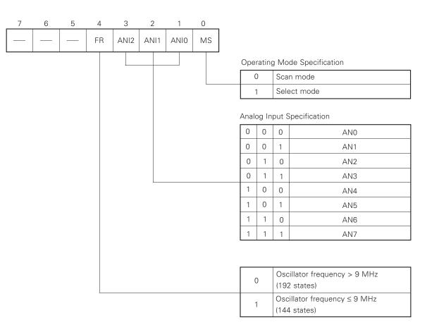
Fig. 2-31 A/D Channel Mode Register Format
