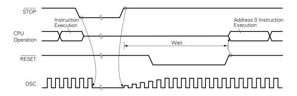
In the case of a hardware STOP mode release, as with a release of the software STOP mode by means of the RESET signal, it is possible to differentiate between a power-on start and a start due to release of the hardware STOP mode by testing the SB flag using a skip instruction.
