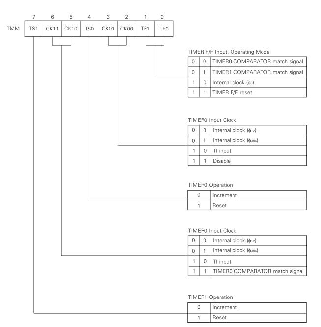
Fig. 2-16 Timer Mode Register (TMM) Format
