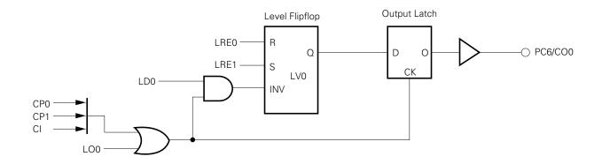
Next, the operation which outputs a square wave to the CO0 pin is described.
