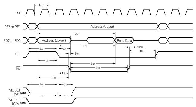
Notes 1. When MODE1 pin is pulled up, M1 signal is output to MODE1 pin in the 1st OP code fetch cycle.
