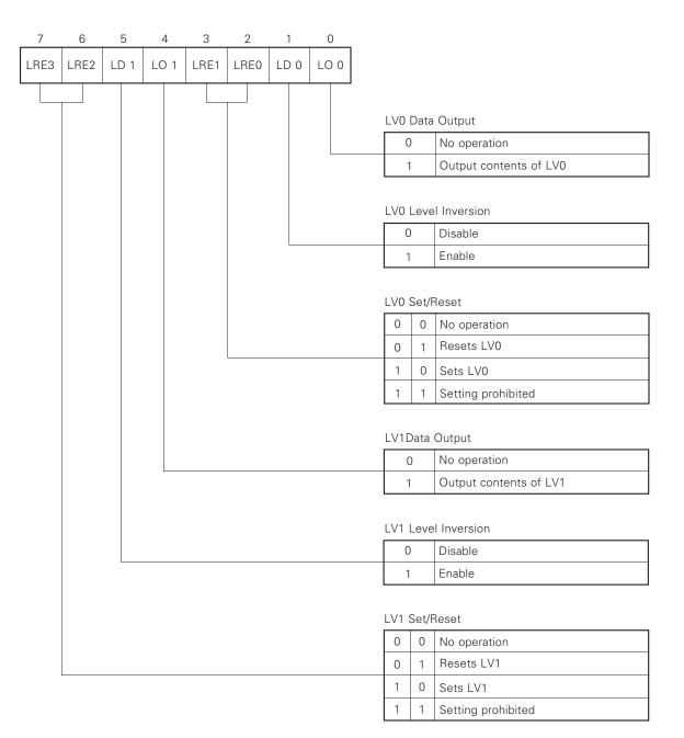
Fig. 2-22 Timer/Event Counter Output Mode Register (EOM) Format
