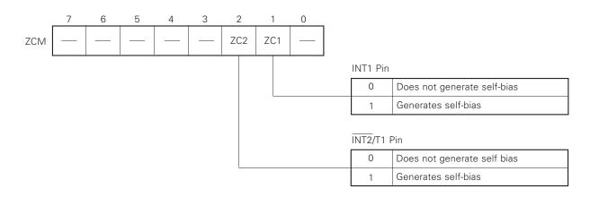
Fig. 2-34 Zero-Cross Mode Register Format
