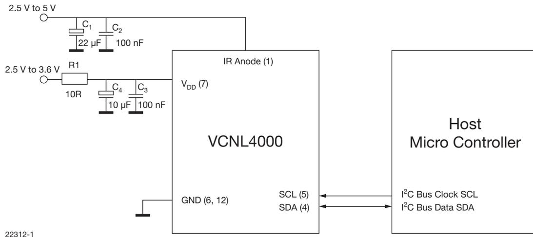
Fig. 12 - Application Circuit
