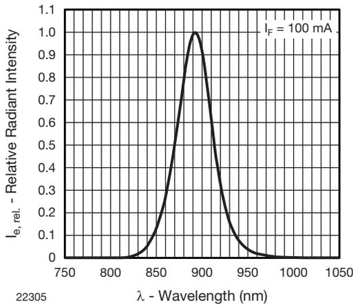
Fig. 5 - Relative Radiant Intensity vs. Wavelength
