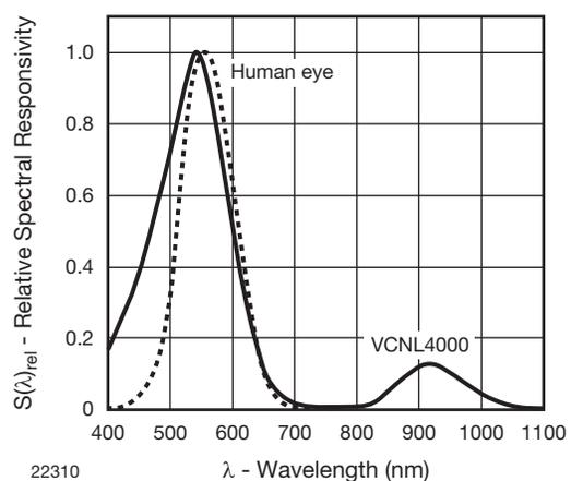
Fig. 10 - Relative Spectral Sensitivity vs. Wavelength
