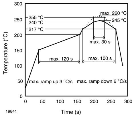
Fig. 19 - Lead (Pb)-free Reflow Solder Profile acc. J-STD-020
