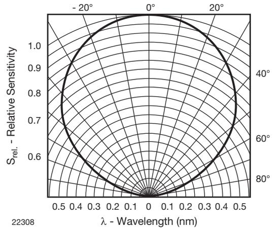
Fig. 8 - Relative Radiant Sensitivity vs. Angular Displacement
