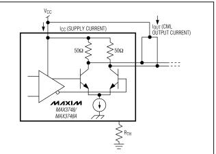
Figure 1. Power-Supply Current Measurement
