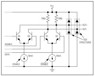
Figure 4. CML Output Buffer
