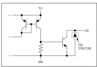
Figure 5. MAX3748 LOS Output Circuit
