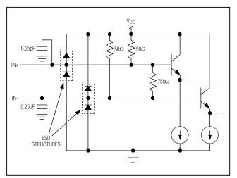
Figure 3. CML Input Buffer
