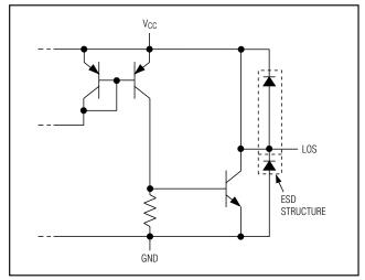
Figure 6. MAX3748A LOS Output Circuit
