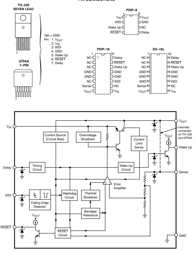
Figure 1. Block Diagram
