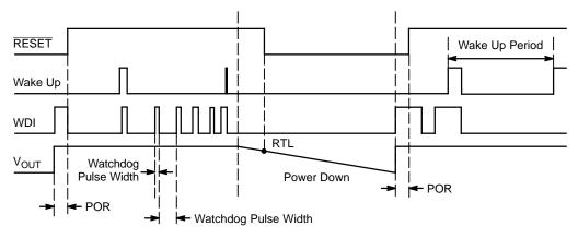
Figure 4. Power Down and Restart Sequence
