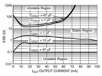
Figure 11. CS8151 Output Stability with Output Capacitor Change
