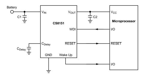
Figure 10. Application Diagram
