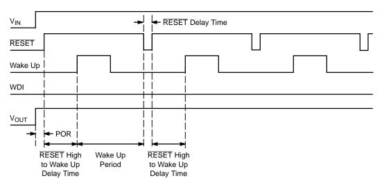
Figure 3. Error Condition: Watchdog Remains Low and a RESET Is Issued
