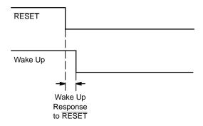
Figure 6. Wake Up Response to RESET (Low Voltage)
