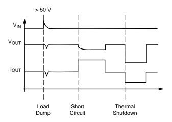
Figure 7. Typical Circuit Waveforms for Output Stage Protection
