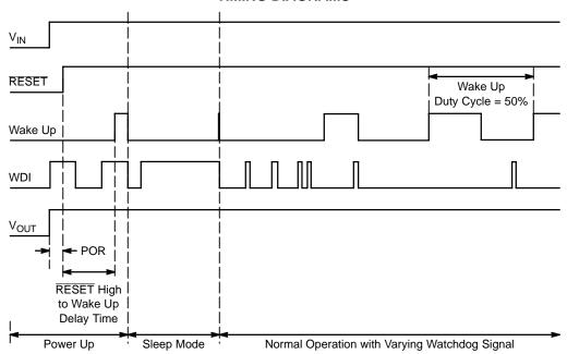
Figure 2. Power Up, Sleep Mode and Normal Operation
