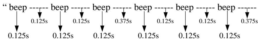
for 4 sec, if the temperature is less than 37.6 ( or 99.6 ) the buzzer will alarms as follows :
