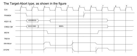
The condition is the target requires the transaction to be terminated and does not want the transaction tried again. As shown in the figure, the DEVSEL# is deasserted when STOP# is asserted. If there is a data needed to be transferred, DEVSEL# must be asserted for one or more clock cycles and TRDY# must be deasserted before target-abort can be signaled.
