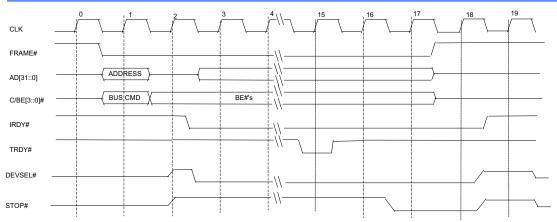
Because W89C940 don't support memory command in burst mode. When the host try to send memory command in burst mode, the first data phase is completed. TRDY# and IRDY# are deasserted, but the FRAME# is asserted for the next data phase. The device will assert STOP# to terminate the transaction. Data is not transferred after STOP# is asserted. The host need to initiate another transaction for further data transfer. The timing is shown above.
