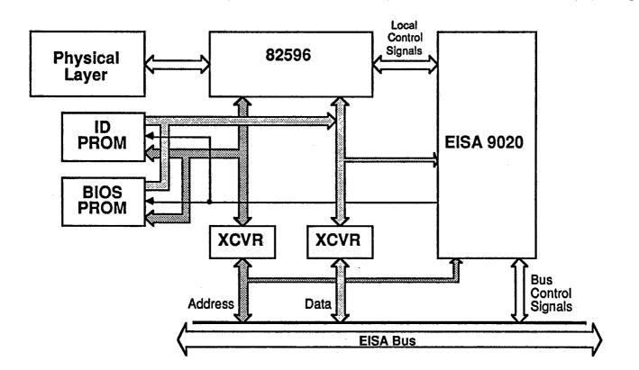
FIGURE 1. Typical Adapter Block Diagram
