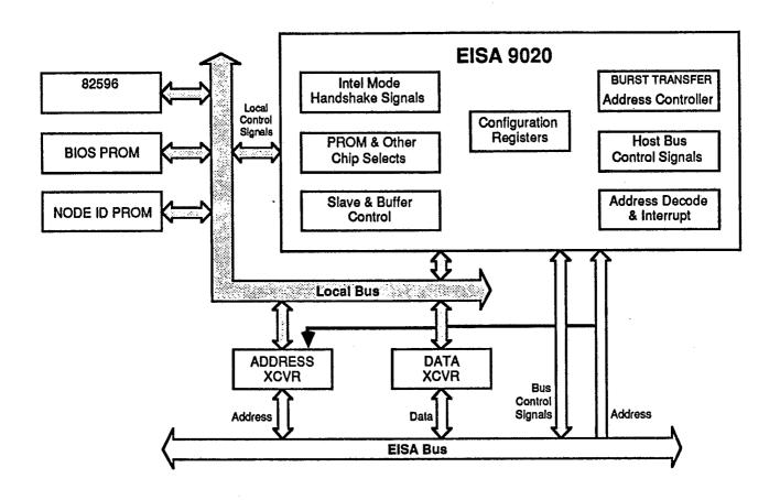
FIGURE 2. EISA 9020 Functional Block Diagram
