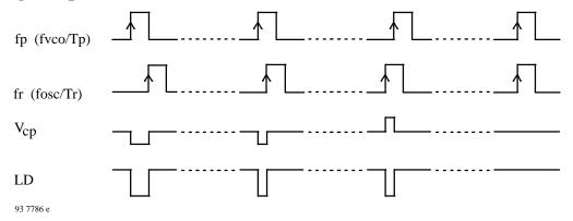
The LD output is in unlocked condition at low level and the pulsewidth is in reference to the phase respectively frequency difference at the phase detector. If the phase detector output pulses are smaller than 100 ns the LD output goes high and indicates "lock" condition.
