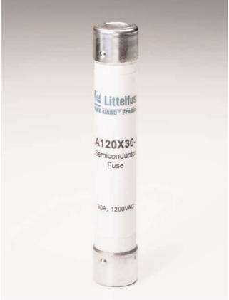
Littelfuse's LA120X semiconductor protection fuses, rated 1/2 through 30A, 1200 VAC are popular for use in traction drive auxiliary circuits and similar applications. LA120X fuses are also suitable for use on 1000VDC auxiliary circuits with low time constants.
