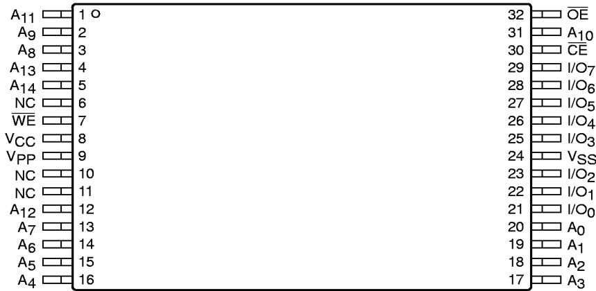
TSOP Package (Standard Pinout 8mm x 14mm) (T14)
