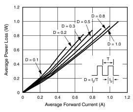
Figure 2. Forward Power Loss Characteristics
