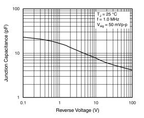
Figure 5. Typical Junction Capacitance
