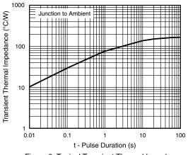
Figure 6. Typical Transient Thermal Impedance
