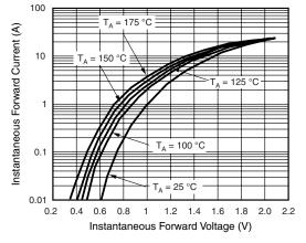
Figure 3. Typical Instantaneous Forward Characteristics
