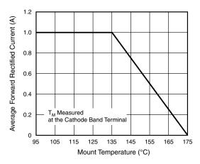
Figure 1. Maximum Forward Current Derating Curve
