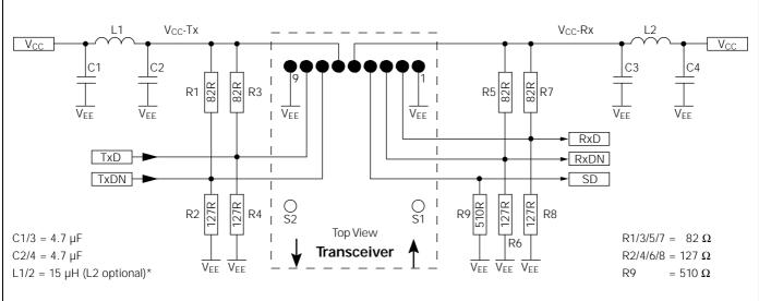
\* Recommended choke is Siemens Matsushita B78108-S1153-K or B78148-S1153-K (Q<sub>min</sub>=60, max. DC resistance=0.6 Ω).
