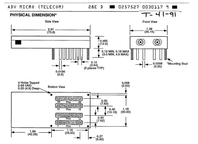
\*Printed Circuit Board mounting included: (mounting studs shown for reference only) 4 Each 2-56 UNC x .635 Long Studs 4 Each 2-56 Nuts
