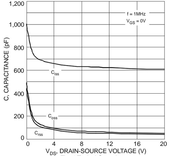
Fig. 4 Typical Capacitance
