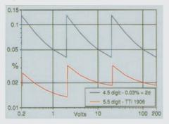
The diagram shows how the effective accuracy varies with reading after taking into account the fixed errors. Over a range of voltages, the 1906 is around four times more accurate than a typical 41/2 digit meter.
