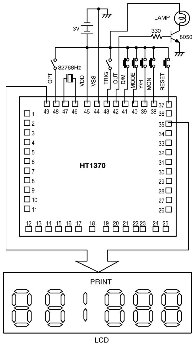
\* The IC substrate should be connected to VDD in the PCB layout artwork.
