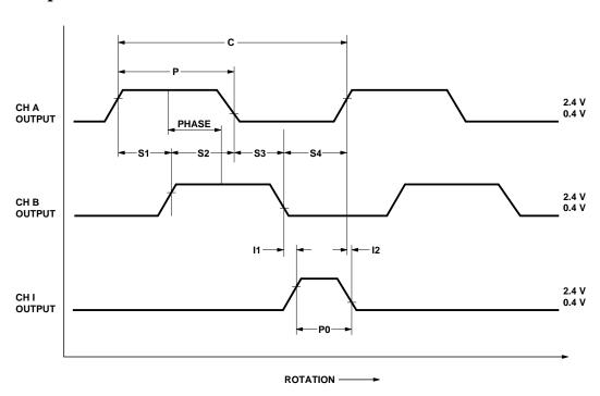
**Waveforms for Encoders without Line Drivers.**
