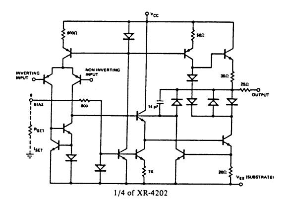
**EQUIVALENT SCHEMATIC DIAGRAM**
