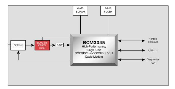
Broadcom's **BCM93345** QAMLink Cable Modem Reference Design is a complete implementation of a certifiable, low-cost DOCSIS/EuroDOCSIS cable modem. The **BCM93345** design is based on the high-performance BCM3345 QAMLink Single Chip Cable Modem and BCM3415 Digital Cable Tuner. The reference design supports both Ethernet and USB interfaces.
