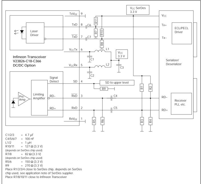
3.3 V-Transceivers can be directly connected to SerDes-Chips using standard PECL Termination network.
