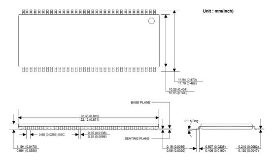
**Note**: Package do not mold protrusion. Allowable protrusion of both sides is 0.4mm.
