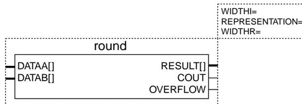
The concept of rounding binary digits is the same as rounding decimal digits. If the digit to the right of the decimal point is greater than 0.5, round the digit up; otherwise, round the digit down. For example, rounding the decimal number 1.25 (01.01<sub>B</sub>) yields 1 (01<sub>B</sub>), and rounding the decimal number 1.75 (01.11<sub>B</sub>) yields 2 (10<sub>B</sub>).
