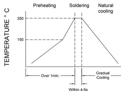
Figure 2. Iron Soldering
