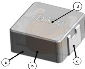
(a) Core : Magnetic metal powder or equivalent
