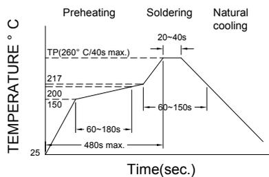
Figure 1. Re-flow Soldering
