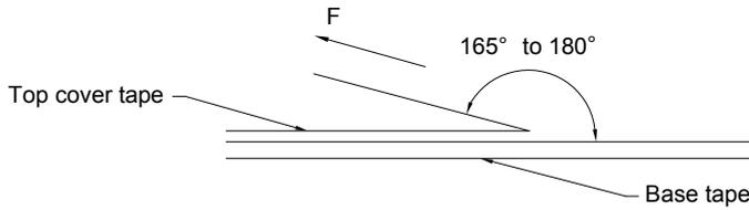
The force for tearing off cover tape is 10 to 130 grams in the arrow direction under the following conditions. (referenced ANSI/EIA-481-C-2003 of 4.11 standard)
