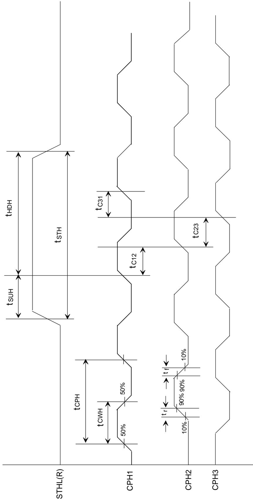
Fig.2 Sampling clock timing
