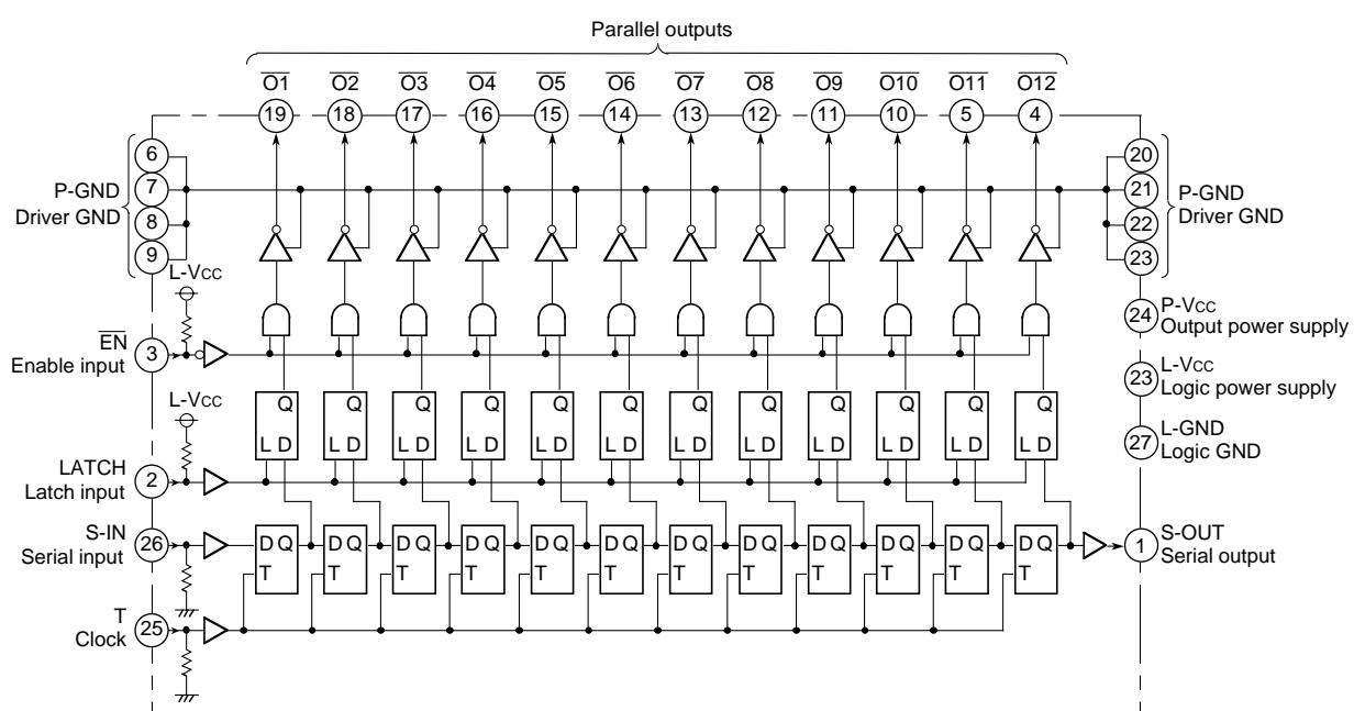
**Bi-CMOS 12-BIT SERIAL-INPUT LATCHED DRIVER**
