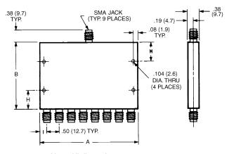
Note: All dimensions are ± .020 except mounting hole diameters (± .005) and mounting hole location (± .010).
