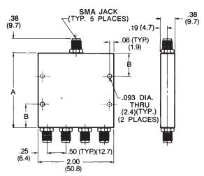
Note: All dimensions are ± .020 except mounting hole diameters (± .005) and mounting hole location (± .010).
