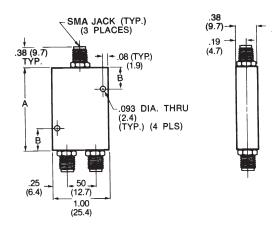
All dimensions are ± .020, except mounting hole diameters (± .005) and mounting hole location (± .010).
