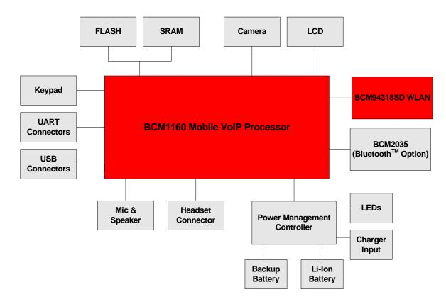
The BCM91160 Wi-Fi Phone Reference Design demonstrates how Broadcom's highly integrated VoIP/WLAN chipset can be used to develop a cost-effective phone for residential and enterprise applications. This chipset is comprised of the BCM1160 Mobile VoIP Processor and the BCM4318 single-chip 802.11b/g baseband, MAC and Radio device.
