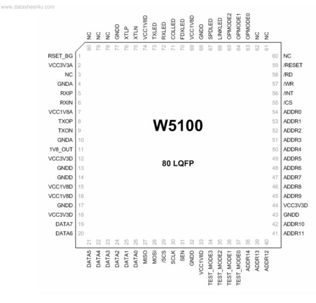
Figure 1. Pinout W5100
