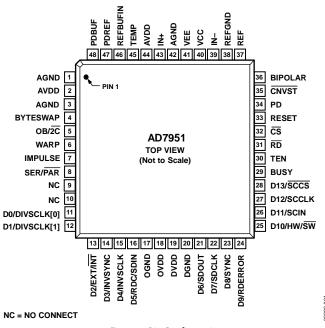
Figure 4. Pin Configuration
