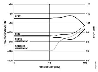
Figure 15. THD, Harmonics, and SFDR vs. Frequency
