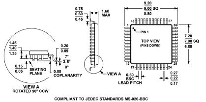
Figure 47. 48-Lead Low Profile Quad Flat Package [LQFP] (ST-48) Dimensions shown in millimeters
