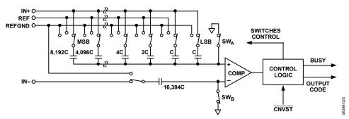
Figure 25. ADC Simplified Schematic
