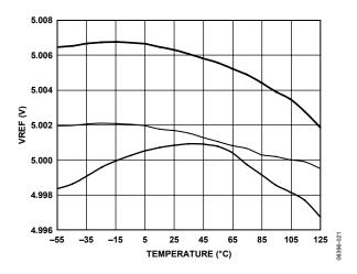
Figure 21. Typical Reference Voltage Output vs. Temperature (3 Devices)
