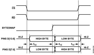
Figure 38. 8-Bit and 14-Bit Parallel Interface
