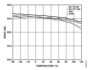
Figure 16. SINAD vs. Temperature
