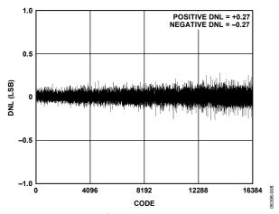
Figure 8. Differential Nonlinearity vs. Code
