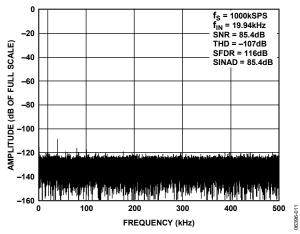
Figure 11. FFT 20 kHz
