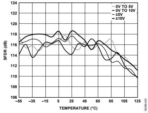
Figure 20. SFDR vs. Temperature (Excludes Harmonics)
