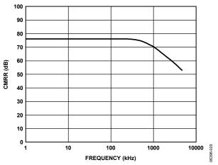
Figure 29. Analog Input CMRR vs. Frequency
