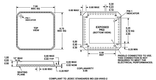
Figure 48. 48-Lead Lead Frame Chip Scale Package [LFCSP\_VQ] 7 mm × 7 mm Body, Very Thin Quad (CP-48-1) Dimensions shown in millimeters
