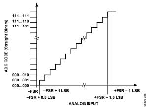
Figure 26. ADC Ideal Transfer Function
