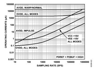
Figure 22. Operating Currents vs. Sample Rate
