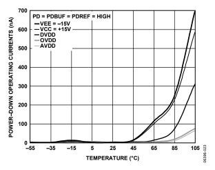
Figure 23. Power-Down Operating Currents vs. Temperature
