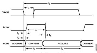
Figure 33. Basic Conversion Timing
