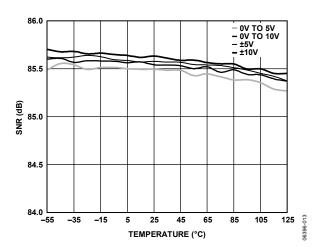
Figure 13. SNR vs. Temperature
