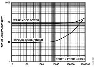
Figure 32. Power Dissipation vs. Sample Rate
