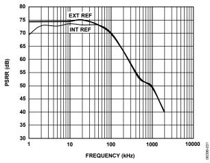
Figure 31. AVDD PSRR vs. Frequency
