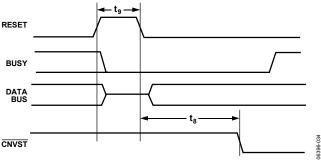
Figure 34. RESET Timing
