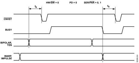
Figure 44. Hardware Configuration Timing
