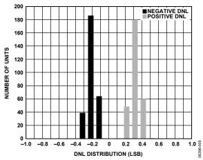
Figure 9. Differential Nonlinearity Distribution (239 Devices)
