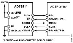
Figure 46. Interfacing the AD7951 to SPI Interface
