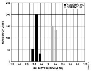
Figure 6. Integral Nonlinearity Distribution (239 Devices)
