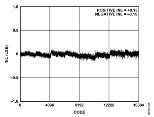
Figure 5. Integral Nonlinearity vs. Code
