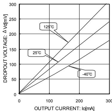
Fig.5 Dropout Voltage ( $V_{cc} = 4.75\text{V}$ ,  $I_o = 0\text{mA} \rightarrow 300\text{mA}$ )
