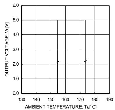
Fig.9 Thermal Shutdown Circuit Characteristics
