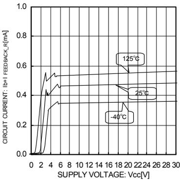
Fig.1 Circuit Current
