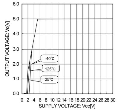
Fig.3 Line Regulation ( $I_o = 200\text{mA}$ )
