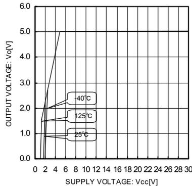
Fig.2 Line Regulation ( $I_o = 0\text{mA}$ )
