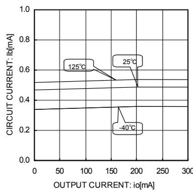
Fig.8 Circuit Current ( $I_o = 0\text{mA} \rightarrow 300\text{mA}$ )
