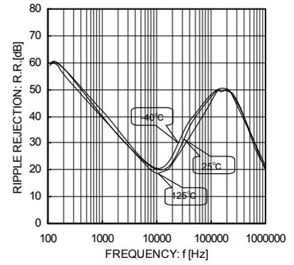
Fig.6 Ripple Rejection ( $I_o = 100\text{mA}$ )
