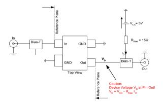
Fig.1: Test Circuit for Electrical Characteristics and S-Parameters
