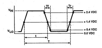
► Duty Cycle 40% to 60% at 1.4V DC level where
