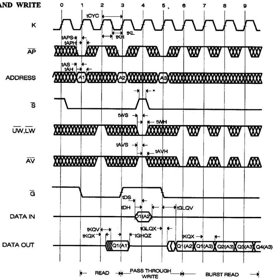
\*The state of  $\overline{S}$  at 4 is ignored due to address A2 being registered one cycle earlier.
