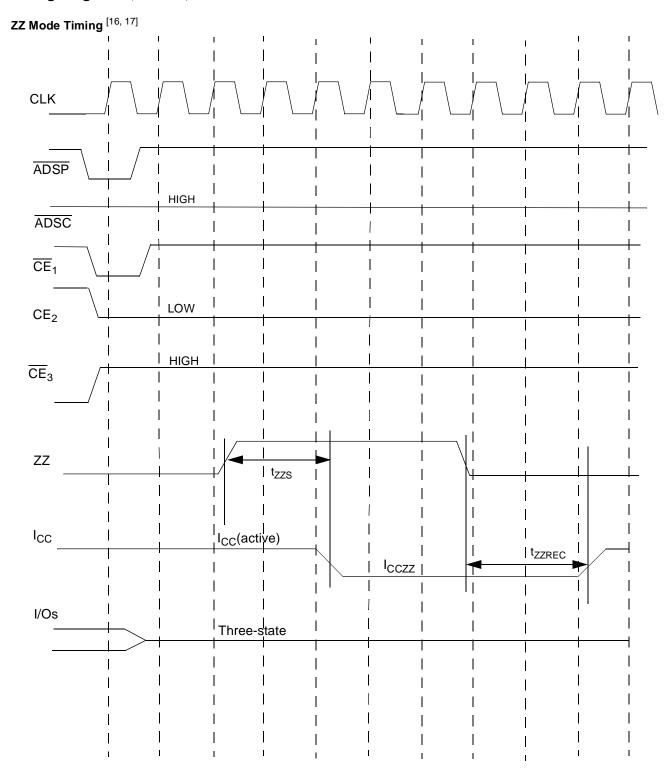
Device must be deselected when entering ZZ mode. See Cycle Descriptions Table for all possible signal conditions to deselect the device.
