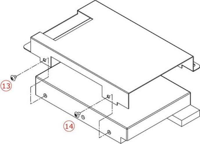
2. When install the HDD, please carefully check the direction of the pin of cable. If wrong direction in use, system fails to function or damage to system will be possible. And it must be connection the HDD cable and HDD power cable then fasten the no.15 ~ no.17 screw to install the drive bay into the chassis.
